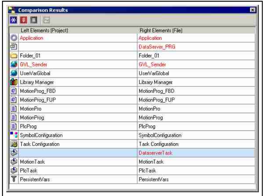
Fig.3-79: Comparison: Application with all subelements with filter option "All elements", "Different elements", "Identical elements"
